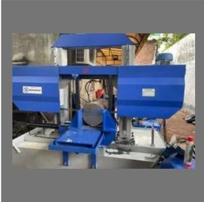
300 To 1000Mm Double Column Metal Cutting Band Saw Machine
