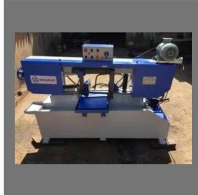
Semi Automatic Metal Cutting Band Saw Machine
