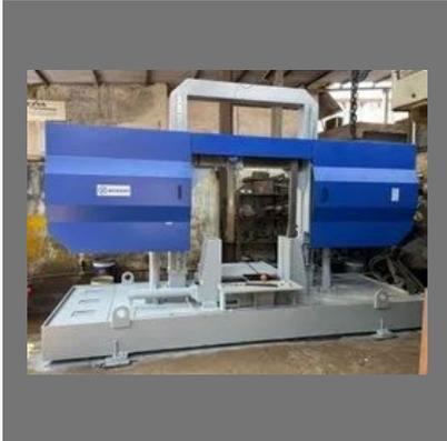
Metal Cutting Double Column Horizontal Band Saw Machine
